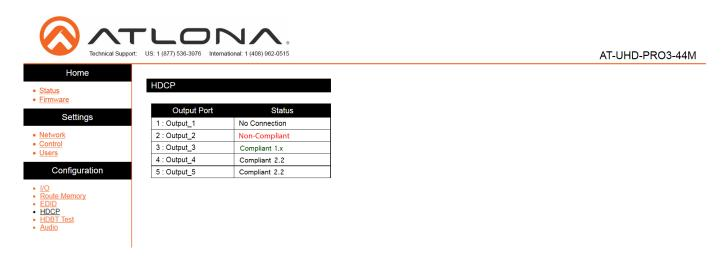
The HDCP page provides a quick way to see whether a display is HDCP compliant or not and the version supported. This page will give multiple status readouts: No Connection, Compliant 1.X, Compliant 2.X, and Non-Compliant.
