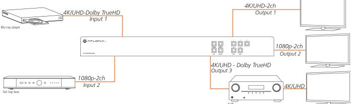
On default, all devices in the diagram will work at 1080p. If a device is not syncing or a different resolution is required, internal EDID or EDID copy and load should resolve these issues. The UHD-PRO3 can copy and store up to 5 EDIDs to memory.
