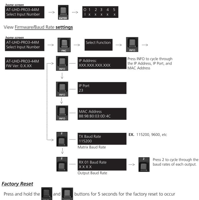
Note: The matrix will not display any signs of the reset. Please wait 5 additional seconds and resume normal operation
