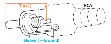
**Note:** Pin outs may vary, please refer to the audio device's manual to ensure a correct connection. **Important!** When terminating cables, please ensure exposed adjacent wires do not touch. This may result in a short that can damage connected devices.
