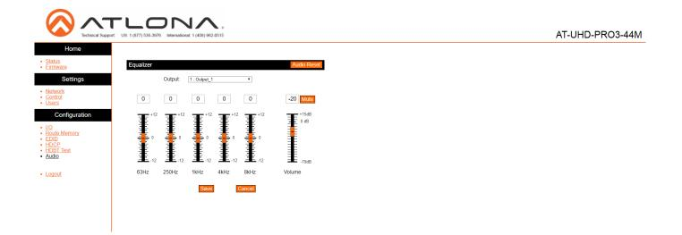
The audio page supports adjustment of 5 band EQ for the analog audio outputs ensuring the best audio performance for each zone. 5 band frequency options at 63Hz, 250Hz, 1kHz, 4kHz, and 8kHz as well as zone output volume and mute.
