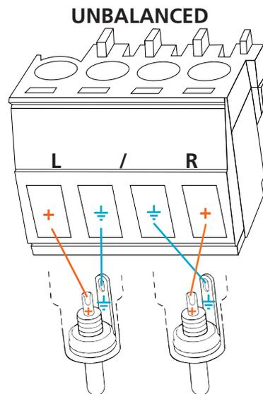
For an easier and time saving solution for analog audio, the optional Atlona Captive Screw Ready 2 Channel Unbalanced Audio Cable (AT-LC-CS-2CH-2M) features pre-stripped wires at one end and RCA connectors at the other end. Purchase these at <http://www.atlona.com>
