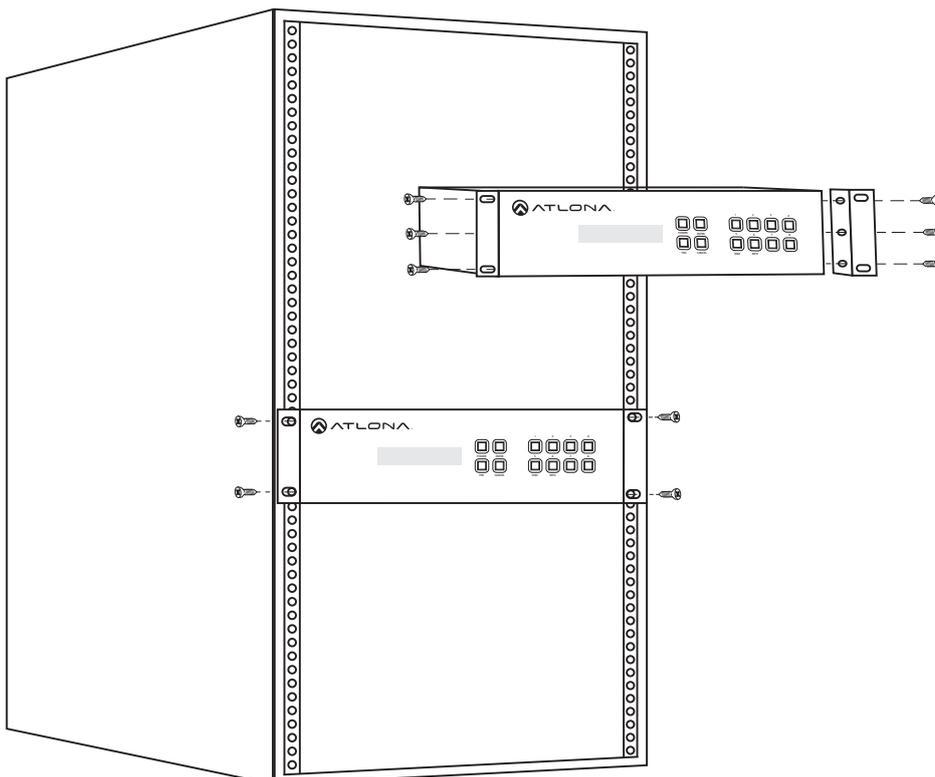
To rack mount the UHD-PRO3 unit: use the rack mount ears, the 6 screws from the sides of the UHD-PRO3, and 4 rack screws.
