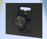
6. If needed the height of the entire bracket assembly can be adjusted by using the notched slots in the key hole plate. Three positions are available. To move the plate loosen the three knobs and move the plate to the desired height then retighten the knobs.
