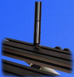
13. Install four camera plate pillars of the appropriate height.
