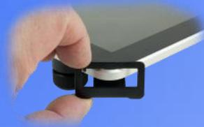
5. Hold in place by positioning the clamps over the corners of the iPad.
