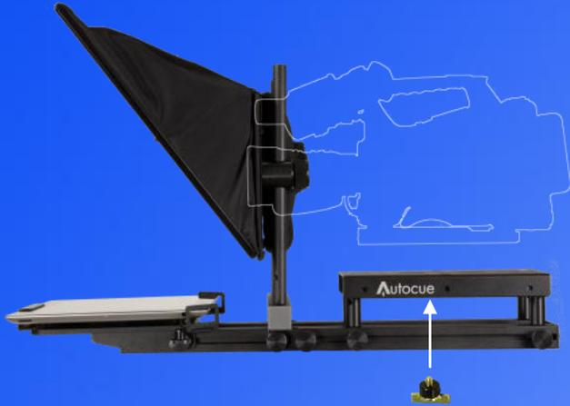
It is important that the camera lens is in the centre of the aperture at the rear of the hood. This is achieved by raising and lowering the camera mounting plate and hood.
