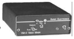
seconds. The adjustment for this timing is set by the Control knob on the front panel. Turn the knob clockwise for a faster fade rate, counter-clockwise for a slower fade rate. The **TAKE** switch controls the fade from either channel A to B, or from channel B to A. Flip the **TAKE** switch towards the channel you wish to fade to. The LED will indicate which channel is currently being displayed.
