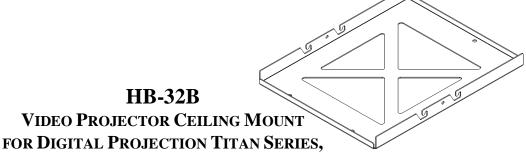
The Chief HB32B video projector ceiling mount is designed to provide fast, simple and secure installation of the Barco CLM10+. Special roll, pitch, yaw and horizontal adjustments simplify projection positioning for image alignment. The HB32B mount also has positive registration lock so that the projector may be removed without losing projector mount registration.
