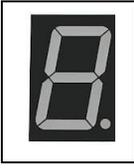
Powering on any DX base station will produce on the LED display the number “8” for approximately 3 seconds.
