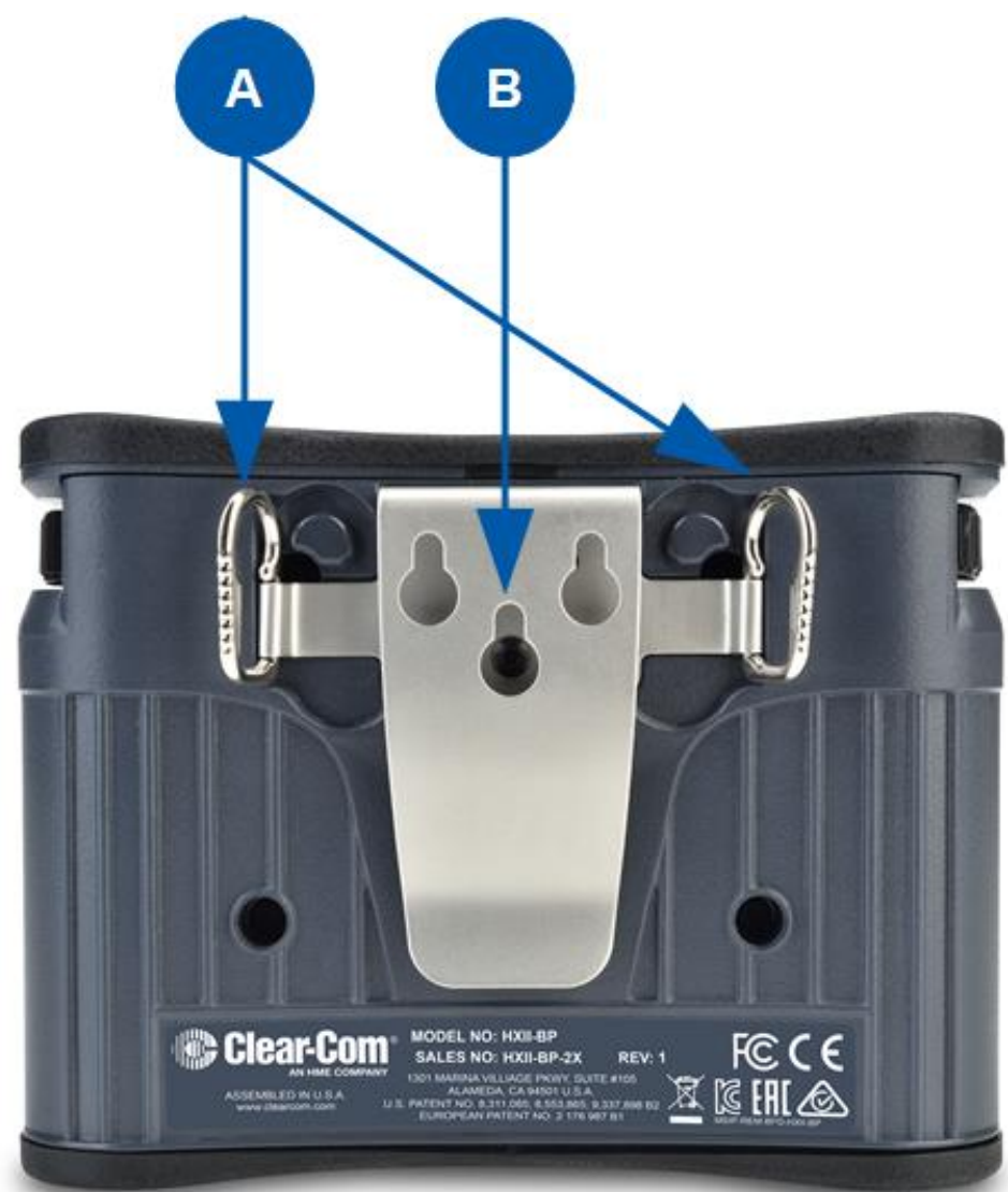
Figure 2-13 HXII-BP-X4 beltloops and clip
