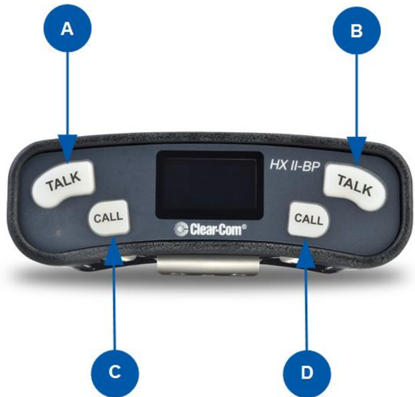
Figure 2-10 HXII-BP-X4 top view
