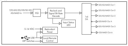
The DA-12G-1x6 can be operated in automatic standard detect mode or in a manual standard mode. Non-inverting ASI reclock is available on **OUTPUT 1** thru **3** and **5** output ports.
