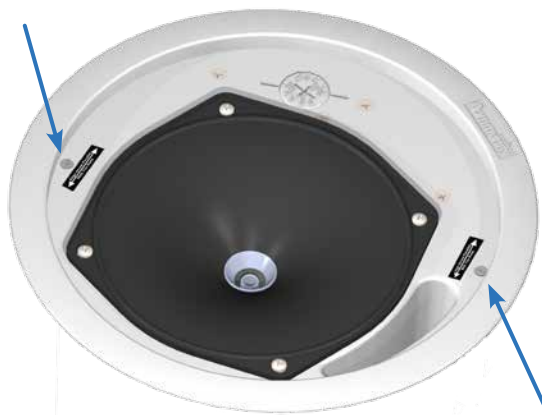
Figure 8. Turning the two loudspeaker clamp actuators clockwise securely locks the unit into the ceiling.
