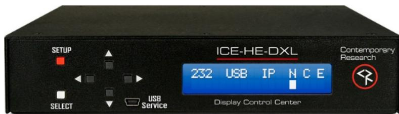
During normal operation, the ICE-HE-DXL displays the above text on the LCD display. The top line shows communication ports as well as network and control status. “Rx” or “Tx” appears briefly under the three external ports (232, USB, IP) to show I/O activity, and a white cursor will blink under the three status options (**N**etwork, **C**ommunication, **E**rror).
