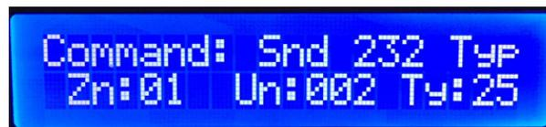
In the **Command** section of the menu above, **Send IR Type** and **Send 232 Typ** are used to match the controllers to the specific TV models and location on the network. There are three parts to the command, selected by moving the **Left/Right** arrows to each value, then using the **Up/Down** arrows to set a number. Press **SELECT** to store the changes.
