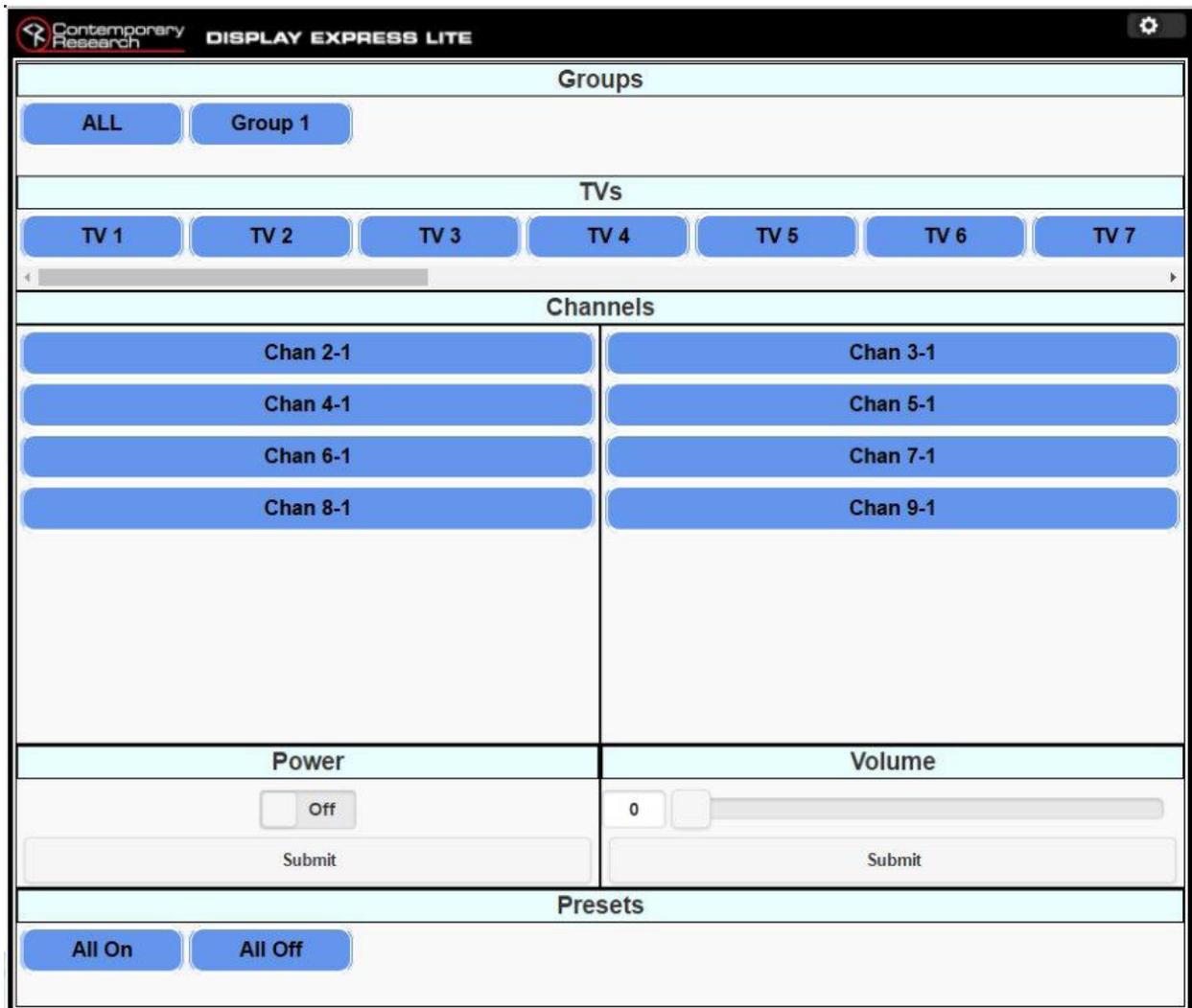
The Display Express Lite web page in the ICE-HE-DXL Display Control Center is a compact version of full Display Express software that runs on a PC. The Lite version is focused on one task – tuning channels for a selected group of TVs, with the added options for TV power and volume, and turning all the TVs on and off.
