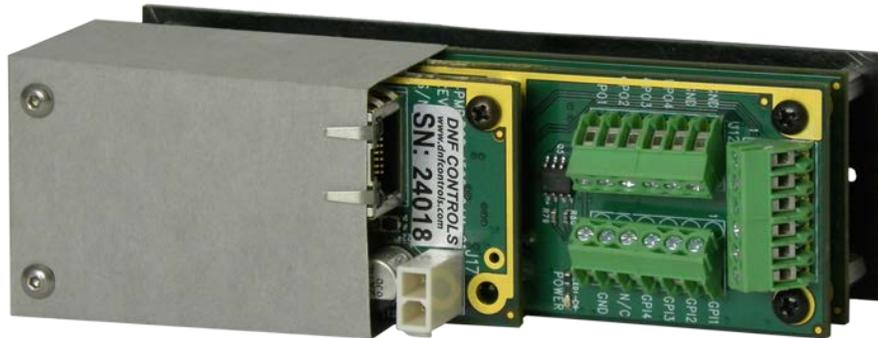
Connect Power Over Ethernet (POE) by inserting Ethernet cable into RJ45 connector on rear. Or, connect external power supply to 2-pin white power connector adjacent to RJ45 connector.
