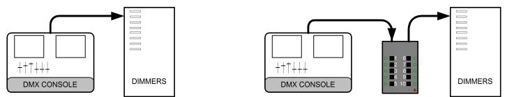
Remove the cable connected to the output of the console. Use a short DMX512 cable to connect the output of the console to the DMX512 input of the *Preset 10 Portable*. Connect the cable that was originally connected to the console to the DMX512 output connector of the *Preset 10 Portable*. This inserts the *Preset 10 Portable* into the DMX512 signal path.
