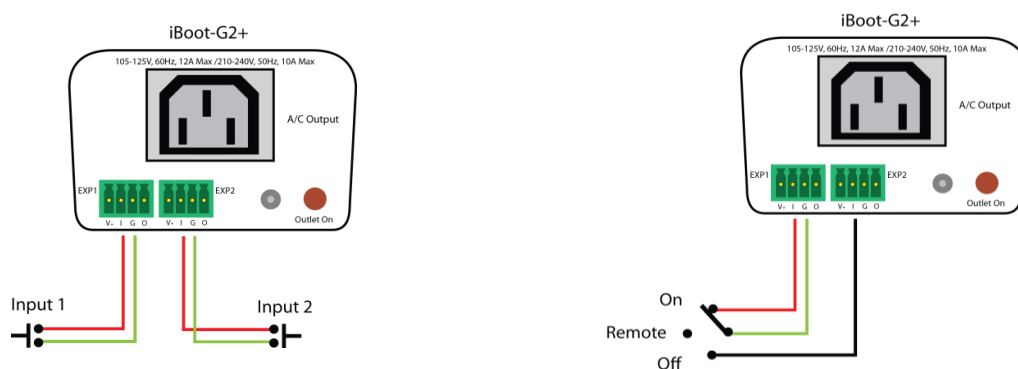
Input Connections to Switches for Power Control
