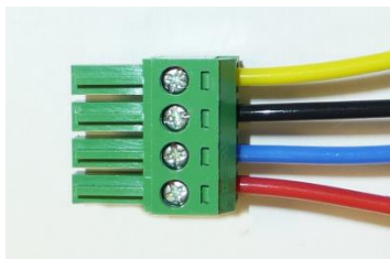
Proper Screw Terminal Connections
