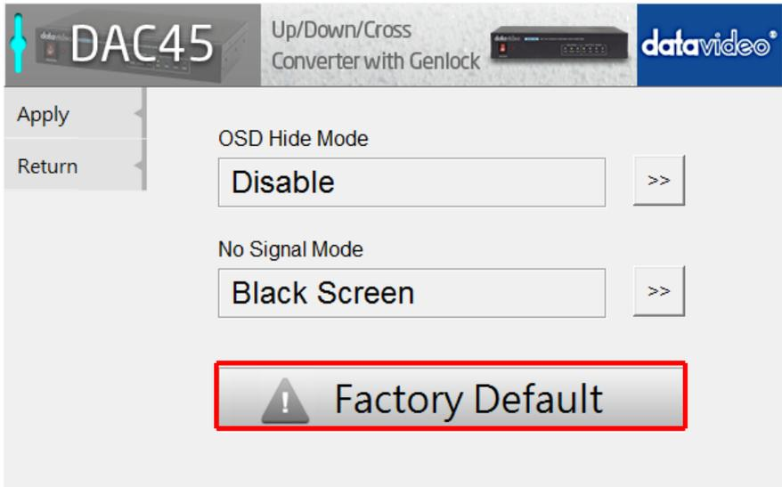
In addition, the user can also set **OSD Hide Mode** and **No Signal Mode**. Details of these two modes are described in the table below.
