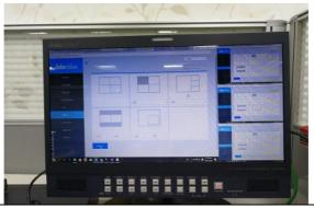
4. PBP (Picture By Picture): Click the PBP icon and select the desired two channels to be PBP and then press the submit button to apply.
