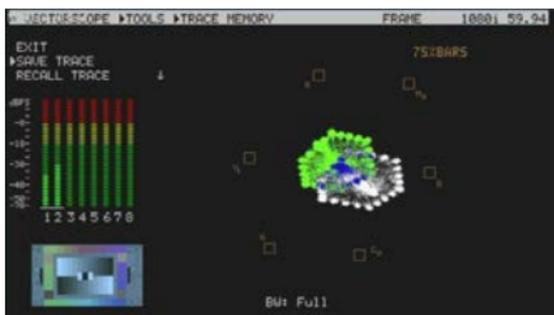
4. Feeding camera output of 75% colour bars into a Video Switcher confirms if the colour image is correct after the switcher too.
