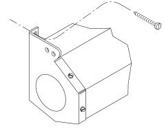
Use the holes at the back of the mounting bracket for flush wall mounting. *Recommended hardware:* For mounting into wood or wall stud, use  $#10 \times 1^{1/4"}$ wood screws; for mounting into drywall (minimum  $^{1/2"}$ thick), use  $^{3}/_{16"}$  toggle bolts or  $^{3}/_{16"}$  molly bolts.
