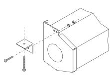
Use the **front** mounting hole in the endcap for recessed mounting flush with the ceiling. Attach angle (not included) to screen then position and properly anchor screw fasteners (not included) into ceiling joists or other solid surface. *Recommended hardware:* For mounting into wood or ceiling joist, use <sup>3</sup>/<sub>16</sub>" bolts.
