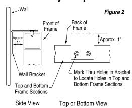
NOTE: Only drill through one side of the frame sections. Holes may need to be deburred.
