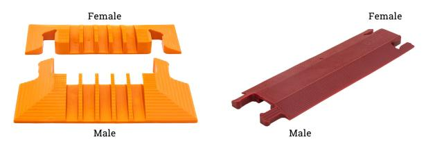
When placing the connection pieces together, always place the female side of top of the male side of the product (see above). Push down on the pieces at the connecting point using your hands or feet. When disconnecting the products, lift the female side upward. This applies to linear pieces, turns and end cap pieces.
