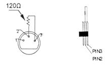
Termination reduces signal errors and avoids signal transmission problems and interference. It is always advisable to connect a DMX terminal, (Resistance 120 Ohm 1/4 W) between PIN 2 (DMX-) and PIN 3 (DMX +) of the last fixture.
