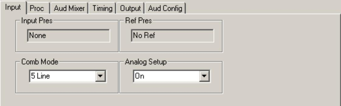
The screenshot shows the 'Input' menu of the BrightEye control application. The menu is divided into six sections: 'Input', 'Proc', 'Aud Mixer', 'Timing', 'Output', and 'Aud Config'. The 'Input' section is active and contains four controls: 'Input Pres' (a text box showing 'None'), 'Ref Pres' (a text box showing 'No Ref'), 'Comb Mode' (a dropdown menu showing '5 Line'), and 'Analog Setup' (a dropdown menu showing 'On').
