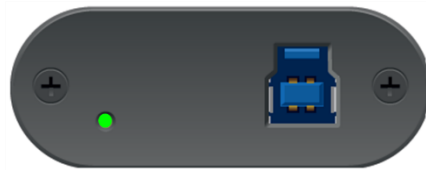
A flashing green LED means USB 2.0
