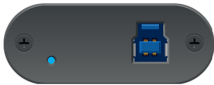
A flashing blue LED means USB 3.0
