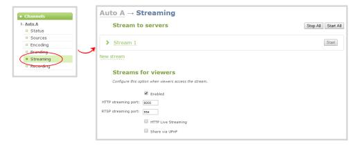
4. Set the **HTTP Streaming port** to specify the port used to stream the HTTP broadcast. This value along with the URL is used by viewers to access the FLV and MPEG-TS streams.
