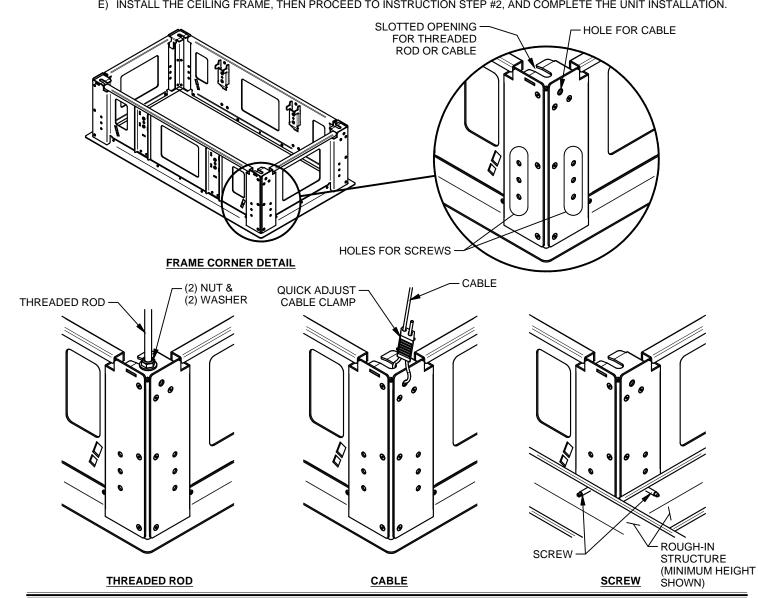
1. INSTALLATION OF THE CB-SR12 CEILING FRAME REQUIRES A ROUGH-IN HOLE IN THE CEILING OF 13" x 25", +/- 1/16". THE HOLE'S
