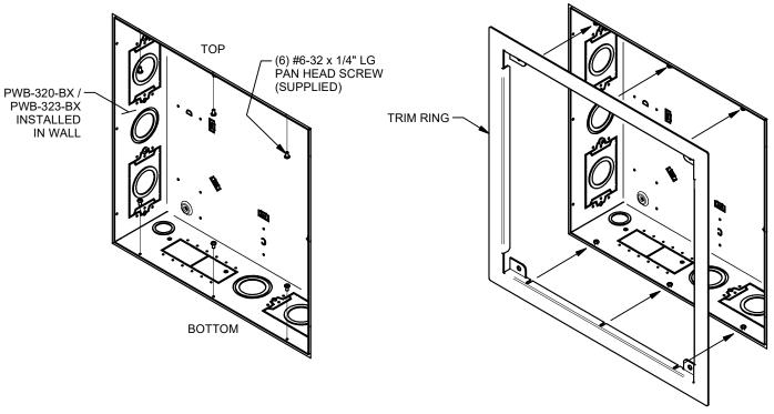
3. PLACE COVER ONTO TRIM RING WITH CABLE EXIT/VENT OPENING TOWARD TOP AND BOTTOM. PRESS IN ON THE SNAP-TOP FASTENERS TO AFIX COVER.
