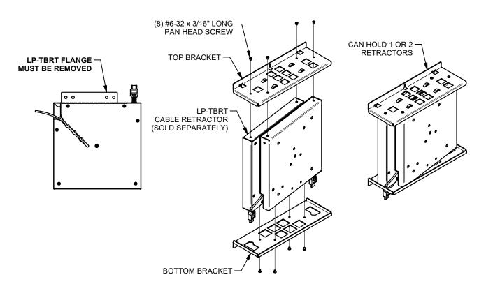
b. HANG RETRACTOR INSIDE BOX AND SECURE WITH #6-32 SCREWS AND MAKE WIRING CONNECTIONS AS REQUIRED.
