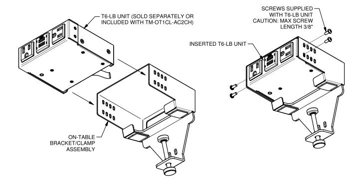
3. LOCATE AND SECURE TO TABLE BY TIGHTENING THUMB SCREW. MAKE ELECTRICAL CONNECTIONS AS REQUIRED.
