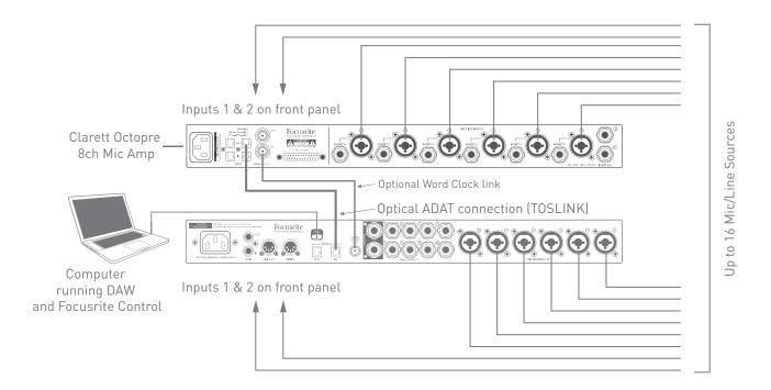
The Clarett OctoPre's **OPTICAL OUT** port is connected to the Clarett 8Pre USB's **OPTICAL IN** port with a single TOSLINK optical cable. Stable word clock synchronisation may be achieved by connecting the Clarett 8Pre USB's **WORD CLOCK** output to the Clarett OctoPre's **WORD CLOCK IN** and setting the Clarett OctoPre to use this as its sync source; alternatively, the Clarett 8Pre USB may be set (in Focusrite Control) to synchronise via the ADAT format signal at the **OPTICAL IN** port.
