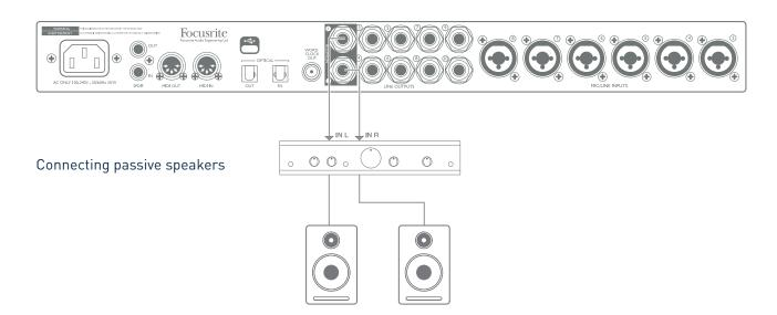
All the line output connectors are 3-pole (TRS)  $\frac{1}{4}$ " jack sockets, and are electronically balanced. Typical consumer (hi-fi) amplifiers and small powered monitors will have unbalanced inputs, either on phono (RCA) sockets, or via a 3.5 mm 3-pole jack plug intended for direct connection to a computer. In either case, use a suitable connecting cable with jack plugs at one end.
