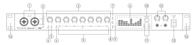
The front panel includes all the input gain and monitoring controls as well as two of the input connectors for Mic, Line and Instrument signals.
