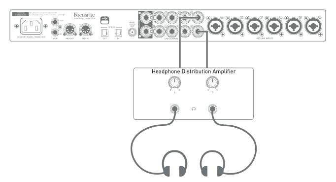
Always remember - when sourcing monitor mixes from input signals, ensure that the DAW channels on which you are recording are muted, otherwise the musicians will hear themselves "twice", with one signal audibly delayed as an echo.
