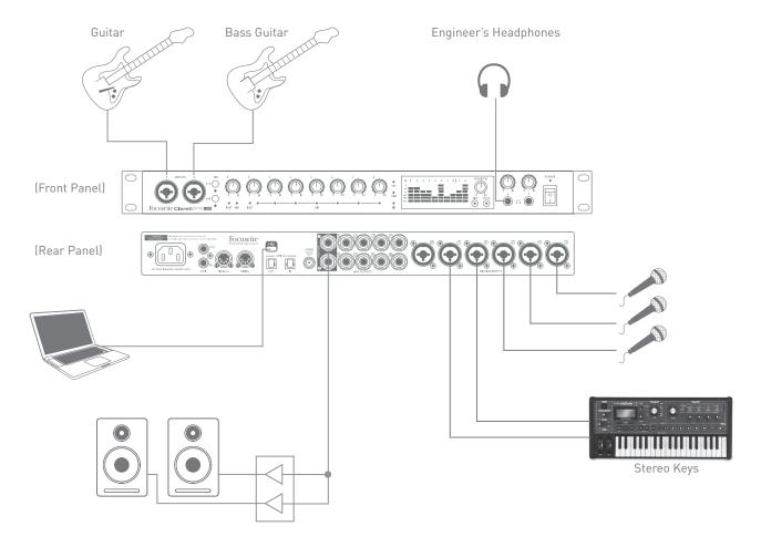
This setup illustrates a typical configuration for multitrack recording with DAW software on your Mac.
