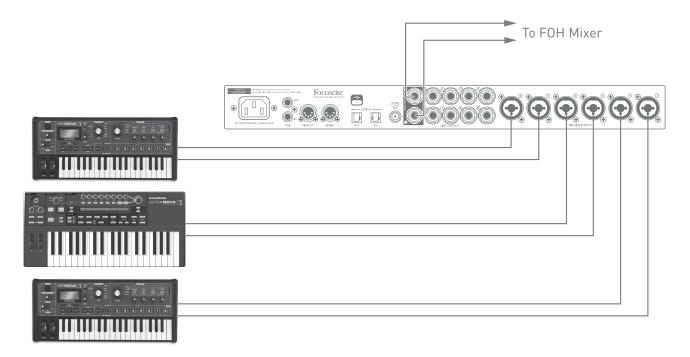
In the example illustrated, three stereo keyboards are connected to the rear panel inputs of the Clarett 8Pre USB; Outputs 3 and 4 go to the main PA system. The performer can adjust the volume of the individual keyboards from the front panel; he/she can also independently adjust the level they hear the mixed keyboards at through the speakers.
