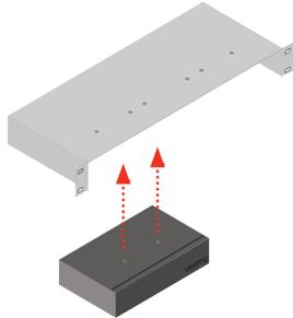
3. Install 2 **flat head, 6-32 thread, 5mm or 3/16" long machine screws** that are either provided with the product or need to be purchased separately (depending on product model).
