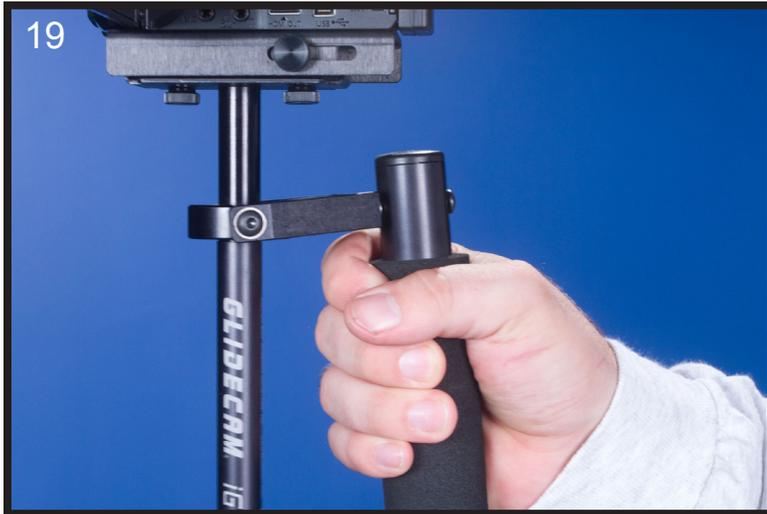
When handling your Glidecam iGlide you will be using one hand to hold onto the handle and the other hand to gently guide the camera in the direction you wish to shoot. We shall call the hand that holds the handle, the holding hand (see photo #19) and the hand that aims the camera for tilting and panning etc the guiding hand. (See photo #20)
