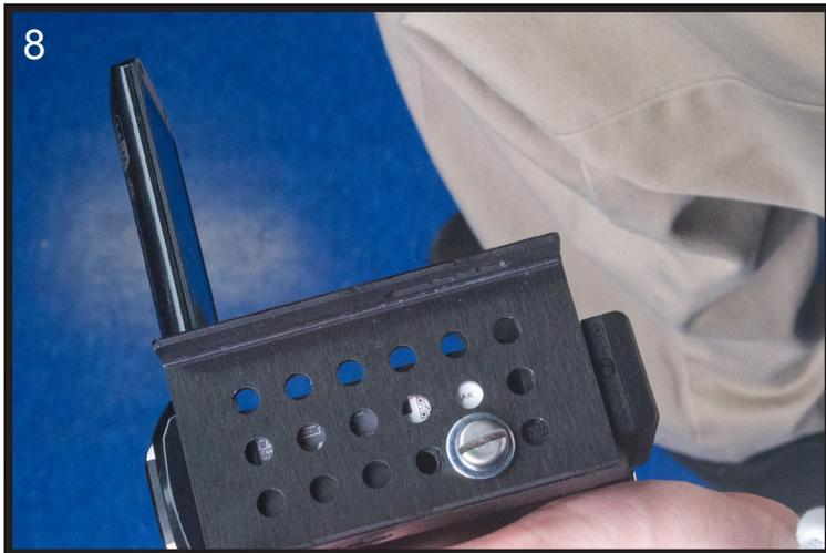
The HEAD PLATE should be secured and square with the camera.
