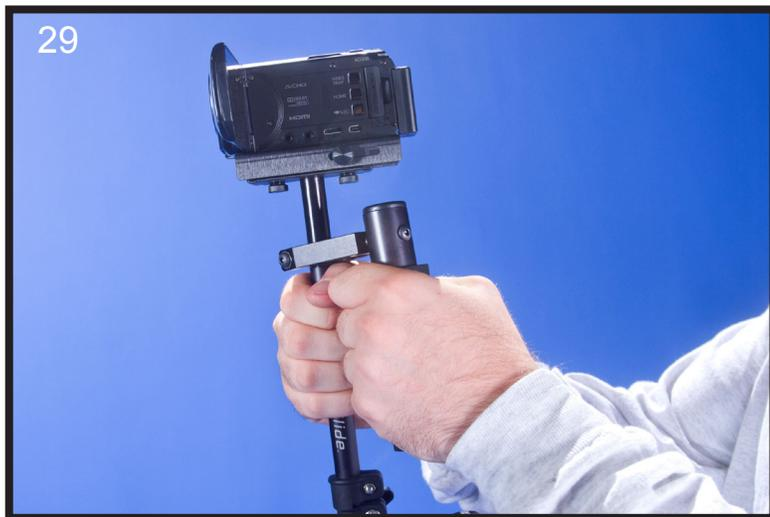
When shooting with the Glidecam iGlide avoid grabbing the **CENTRAL POST**, (see photo #29) this defeats the purpose, and isolation that the three axis gimbal provides. Instead handle your Glidecam iGlide as shown in photo #20
