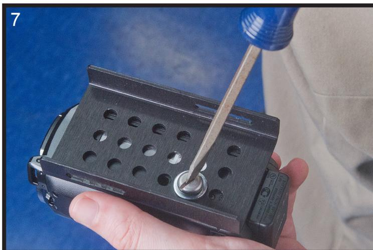
Place your camera upside down in your lap and with the HEAD PLATE in place use a flat head screwdriver to secure the HEAD PLATE to your camera using the CAMERA MOUNTING SCREW you've just selected.
