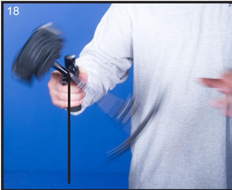
**To test the balance of the vertical axis,** perform what is called the SLED ARC TEST. To perform the “Sled Arc Test” simply hold the iGlide by its handle and grab hold of the back end of the iGlide BASE PLATFORM and pull the base up and back until the iGlide CENTRAL POST is horizontal (see photo #16). Now carefully let go of the BASE PLATFORM and count how many seconds it takes for the iGlide to then first swing to vertical (see photo #17 & #18)
