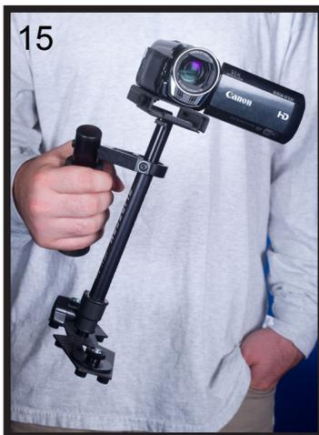
Also, another way of fine tuning the horizontal balance is to move the COUNTER WEIGHT DISKS back and forth, or side to side on the BASE PLATFORM. There are slots on the BASE PLATFORM to help with this task. Also, replacing the WEIGHT DISKS away from the CENTER POST on the BASE PLATFORM will increase panning stability. Make sure to tighten the WEIGHTS down after you move them.
