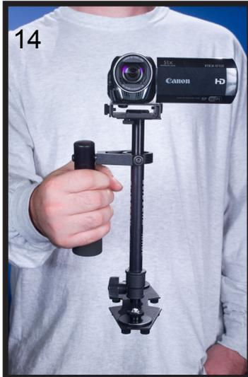
If the iGlide leans to the right, then you will have to loosen up the BLACK THUMB SCREWS on the bottom of the BOTTOM PLATE and gently slide the MID PLATE over to the left a bit. If the iGlide leans to the left, then move the MID PLATE to the right. Always secure and firmly tighten the BLACK THUMB SCREWS after any adjustment.
