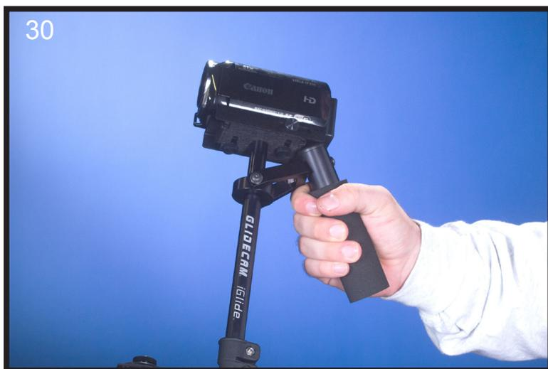
Also, allowing the handle of the Glidecam iGlide to come in contact with the **BOTTOM PLATE** (see photo #30) is something that you should avoid. This limits your range of motion, and will result in "jerky", and unpleasant footage. Instead position the handle as shown in photo #19
