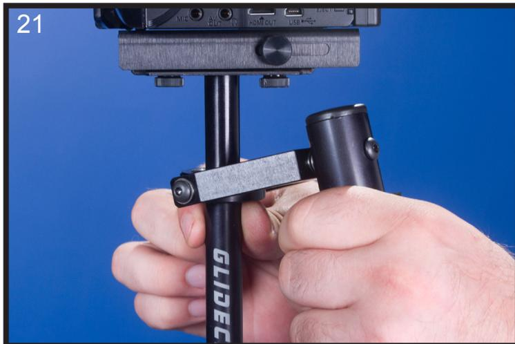
The Glidecam iGlide is designed to work correctly only when operated with two hands. (See photos #19, #20) One being the holding hand and the other being the guiding hand. If you try to operate the unit with just your holding hand, the camera might drift away from its originally balanced set-up position. Also, without the guiding hand in place, you will be unable to control the direction of the camera.
