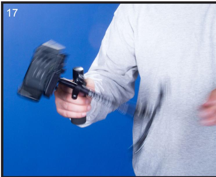
Photo #17 shows the Glidecam iGlide swinging between horizontal and vertical during the "Sled Arc Test" (see next page)
