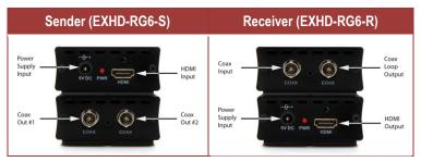
The sender provides one HDMI input and two coaxial BNC output connectors for connection to up to two receivers.
