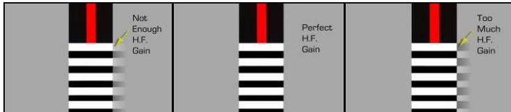
Figure 5 - Effect of adjustment on the smearing
