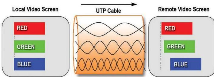
Figure 6 - Skew mechanism
