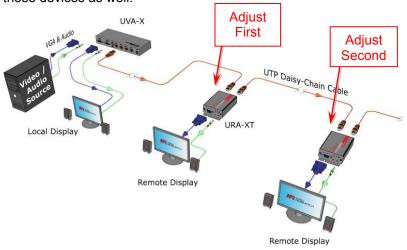
Figure 8 – Daisy-Chain adjustment sequence
