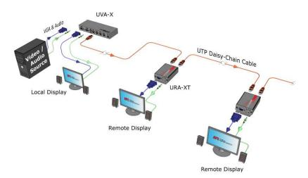
Figure 3 - URA-XT Application Diagram
