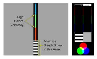
Figure 4 - Typical test patterns used for adjusting compensation
