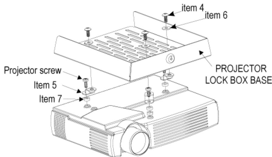
NOTE: Do not over tighten the bracket mounting screws as damage to the projector's internal mounting threads could occur.
