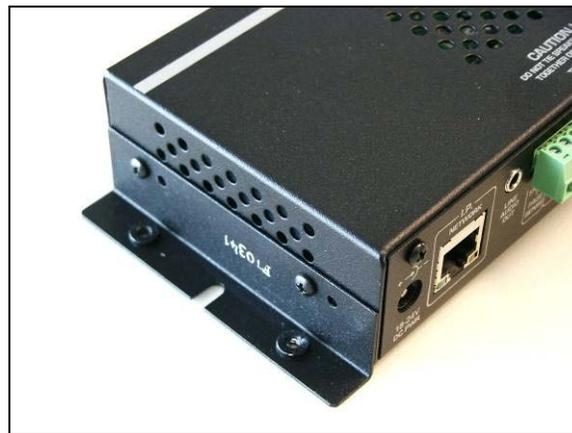
Bracket installation for surface mounting
