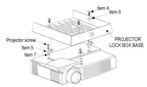
NOTE: Do not over tighten the bracket mounting screws as damage to the projector's internal mounting threads could occur.
