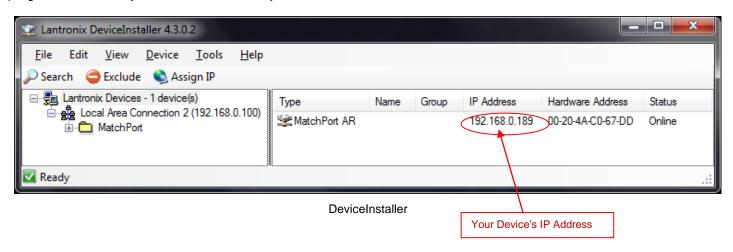
Don't try to change the IP address of your appliance here. The IP address can be changed from Web interface or from Serial interface
