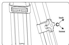
Special Note: It is a best practice to unlock, adjust, and re-lock the tripod legs before the legs are unfolded.
