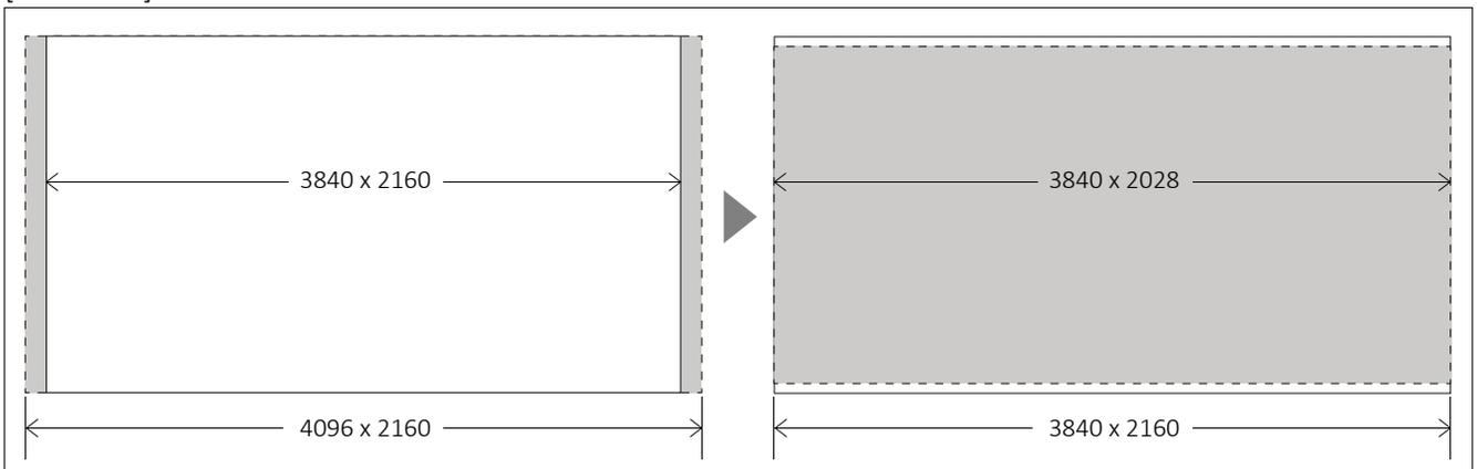
When the 4096x2160 signal is fed, if you select Zero Scan using [Scan] button on the front panel, the picture is scaled to be displayed on the panel of 3840x2048 resolution with maintaining 1.89:1 ratio.
