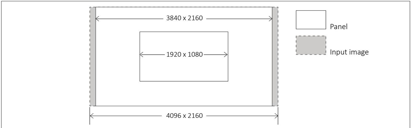
The LCD panel resolution of OBM-U090/U170 is FHD(16:9) 1920x1080. So, when Zero Scan is selected, if the input signal is QHD(3840x2160) it is scaled to 1920x1080(16:9), and if the input signal is DCI 4K(1.89:1) 4096x2160 it is scaled to 1920x1012(1.89:1).
