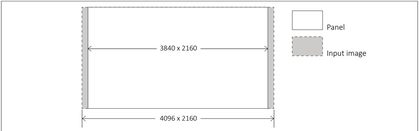
The LCD panel resolution of OBM-U240/U550L is QFHD(16:9) 3840x2160, so if the input signal is 3840x2160, 1:1 mapping is supported. If the input signal is DCI 4K(1.89:1) 4096x2160, 1:1 mapping is not supported.
