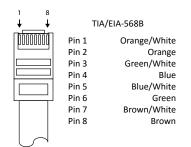
The TCP/IP port requires a standard straight-through Category 5 or greater cable with the TIA/EIA-568B crimp pattern for operation.
