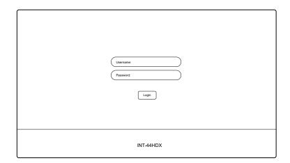
Open a web browser and go to the IP address of the INT-44HDX. The default IP address is 192.168.0.178.
