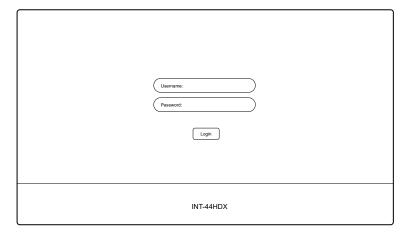
Open a web browser and go to the IP address of the INT-44HDX. The default IP address is 192.168.0.178.
