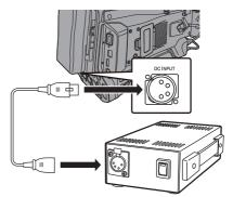
2 Turn on the power of the AC adapter, followed by setting the [POWER ON/OFF] switch of this unit to "ON".
