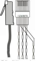
Notice: Cable connectors MUST be metal one, the shielded layer of cable MUST be connected to the connector's metal shell, to make a better transmission.
