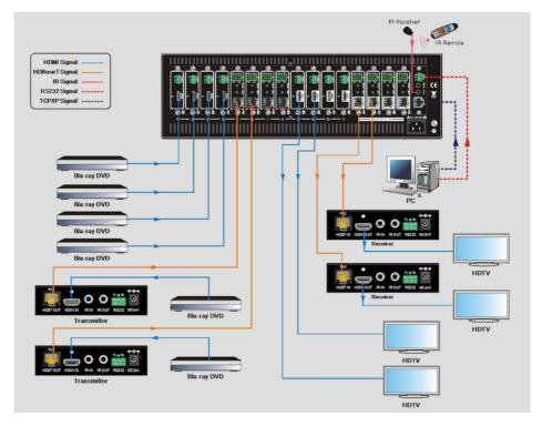
Figure 3-1 Connection Diagram
