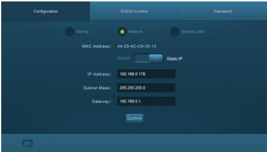
In this interface, dynamic or static IP mode can be selected. Under static IP mode, IP address and subnet mask, gateway can be set and make sure the IP addresses are different to avoid IP conflict.
