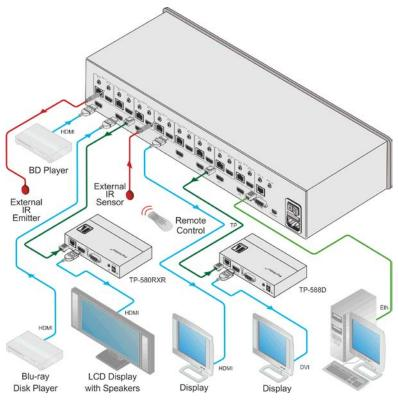
Figure 3: Connecting the VS-88DT HDMI/HDBT Matrix Switcher
