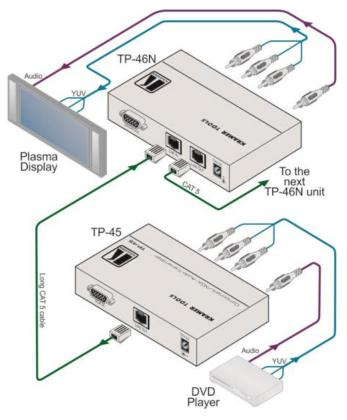
Figure 3: Distribution System, Component Video Mode
