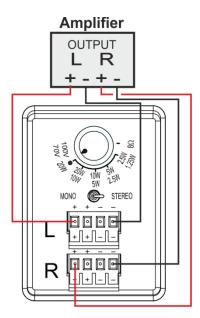
Figure 2: Yarden 6-OD Stereo Setup
