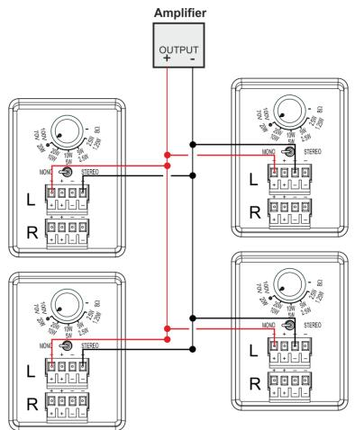
Figure 7: Square Layout Parallel Wiring
