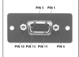
The **WX-MF** is a Male VGA to Female VGA connection module.
